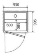
Hole through floor: 930x960 mm Platform: 800x580 mm
