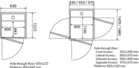
Hole through floor: 930x122 Platform: 800x845 mm Doors: 800 mm Load: 250 kg
